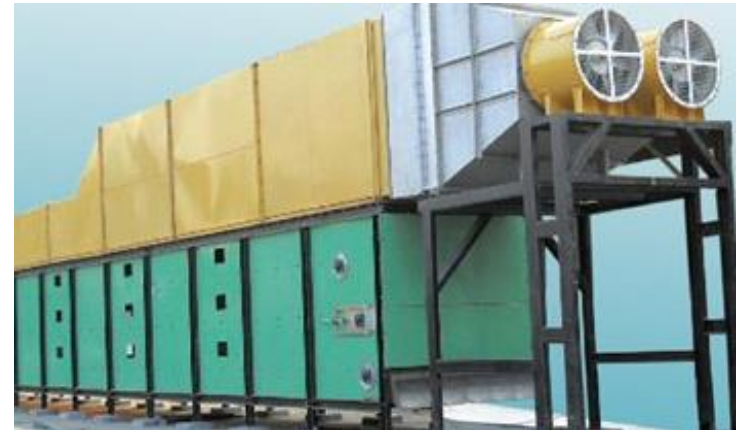
Mechanised Withering System for Tea Leaf
