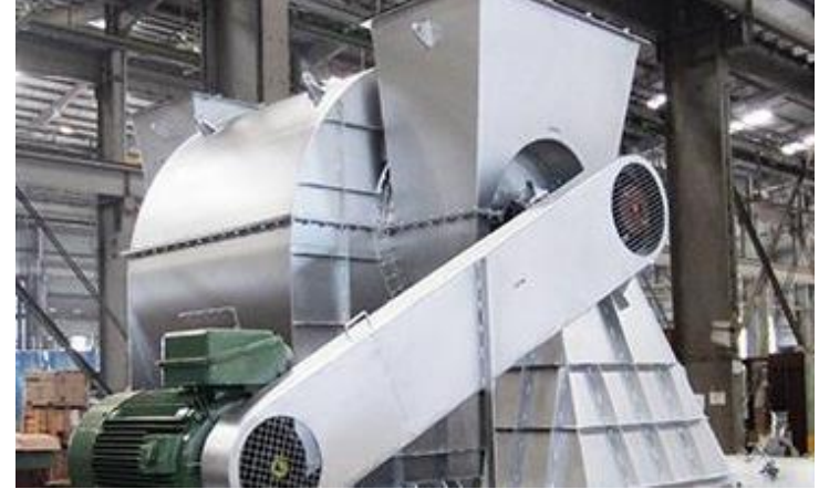
Mechanised Withering System for Tea Leaf
